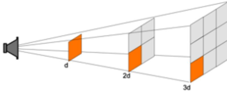
In the case of the gilua-*Tex* cubicle, its design allows the entire surface of the clothing to be kept at a minimum distance from the light emitters, thus maximising the irradiance on the surface and minimising the cleaning cycle for each garment.
